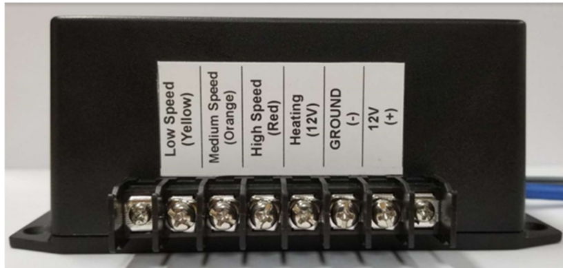
Fig. 26 Control box wiring connections
